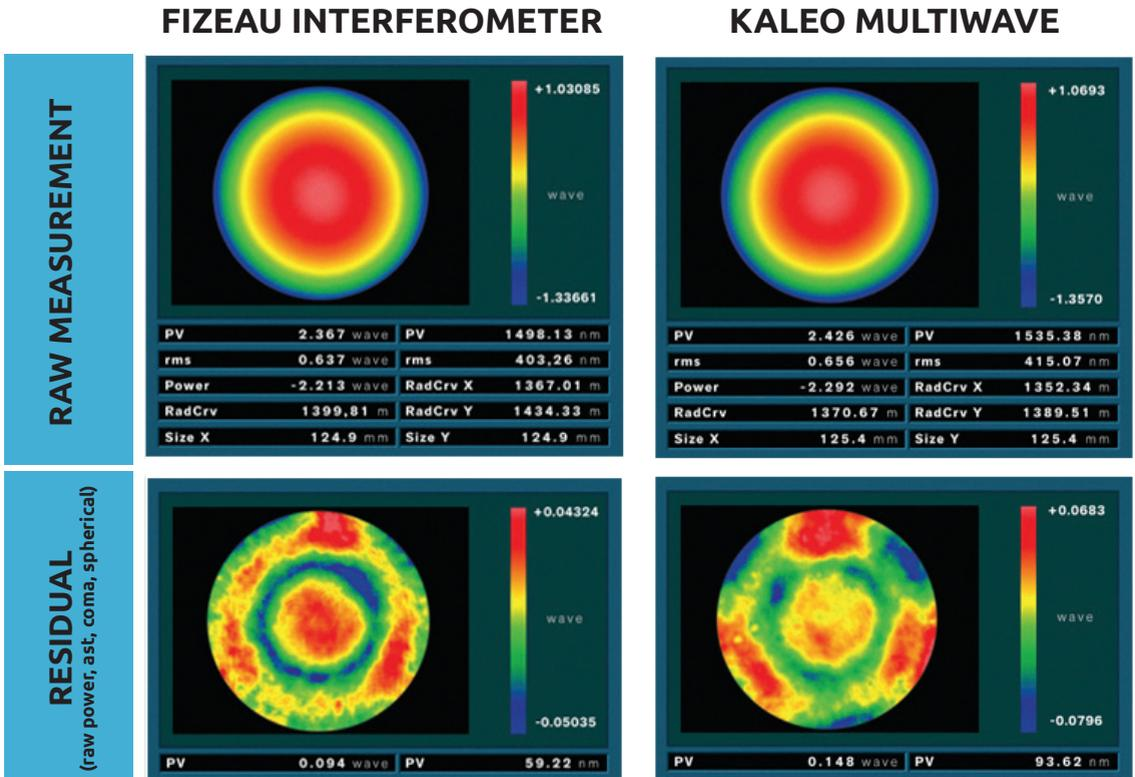
NBP-780nm - The difference between the 2 measurements on the same pupil is below 40
