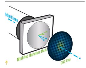
PHASICS technology was introduced to overcome the Shack-Hartmann sensor limitations, especially resolution. This ultra-high resolution enables accurate wavefront measurement for robust calculations of beam parameters.
