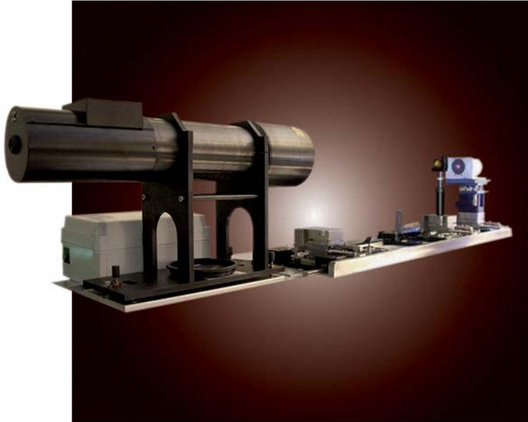
→ PHASICS creates the revolution in **infrared optics quality control** with the Kaleo Bench-IR series. These innovative benches offer both **MTF and wavefront quality** (aberrations, WFE) in **one single fast acquisition**. They cover the full IR range from **1.2  $\mu\text{m}$  to 14  $\mu\text{m}$** .
