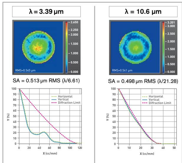
*Chromatic behaviour measured with one unique sensor on a ZnSe lens of 25.4 mm diameter. The focal spot shifts 560  $\mu\text{m}$  due to refractive index dispersion.*
