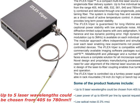
The iFLEX-Viper™ is a compact multi-line laser source with a modular singlemode fiber delivery system. Up to five individual lasers (selected from the range 405, 445, 488, 532, 561, 640 and 780nm) are efficiently combined and delivered through one singlemode, polarization maintaining fiber. The system is mode-hop free and wavelength stabilized as a direct result of active temperature control. A closed loop control provides long term power stability.
